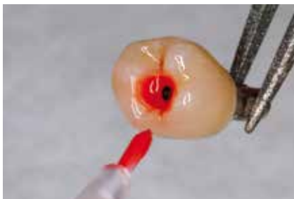
The screw channel is etched from the occlusal side with 5% hydrofluoric acid gel (IPS ® Ceramic Etching Gel) for 20 seconds.
